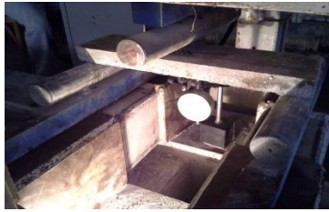
Figure (1) Flexure Test of Reinforced Laminates
