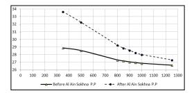
Figure (9) The Temperature at El-Ain-Al Sokhna Intake for different pipe lengths
