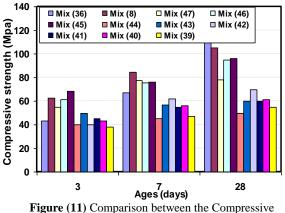
Strength and the Ages for the Concrete Mixes Contained different Types of Aggregates
