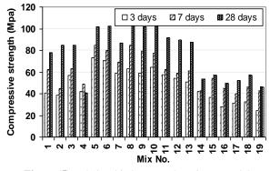
Figure (5) Relationship between the Mix No. and the Compressive Strength for the Mixes Contain different Percentages of Silica Fume Mixes without Superplasticizer
