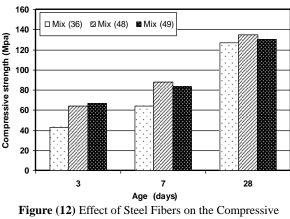
Figure (12) Effect of Steel Fibers on the Compressive Strength
