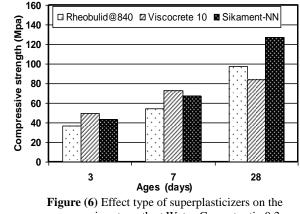
compressive strength at Water-Cement ratio 0.3
