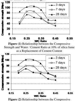
Strength and Water / Cement Ratio at 15% of Silica fume as a Replacement of Cement Content
