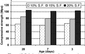
**Figure (4)** Relationship between the Compressive Strength of Different Percentages of Silica Fume as a Replacement of Cement Content at 0.3 W/C Ratios.
