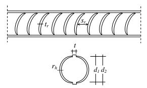
Figure 2. Geometry of the steel bars
