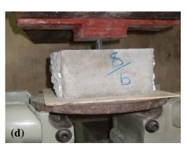
Figure 4. Preparation and testing of push-out test specimens
