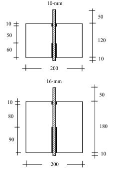
Figure 3. Configuration of push-out bond test specimens
