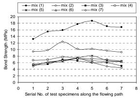
Figure 6. Bond strength along the flowing path (10-mm bar diameter specimens)
