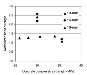
Figure 5. Normalized bond strength and corresponding compressive strength
