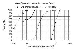
Figure 1. Particle size distribution for concrete materials
