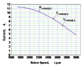
Fig. (11) Motor current-rotor speed characteristics for voltage, resistance and reactance variation.
