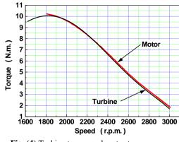
Fig. (4) Turbine torque and motor torque versus rotor speed when the applied voltage is changed.
