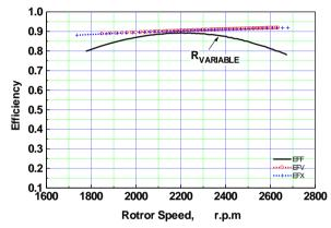
Fig. (16) Efficiency-speed characteristics for voltage, resistance and reactance variation.
