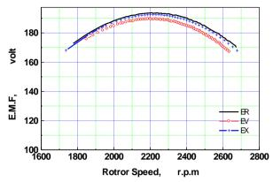
Fig. (15) Induced e.m.f.-speed characteristics for voltage, resistance and reactance variation.
