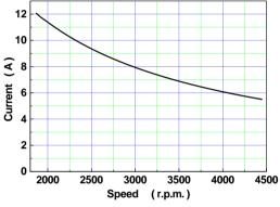
Fig. (3) Motor current variation with rotor speed
