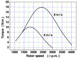
Fig. (1) Turbine torque variation with speed after gear box
