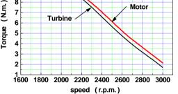
Fig. (8) Turbine torque and motor torque versus the rotor speed for adding resistance.
