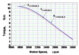
Fig. (10) Torque-speed characteristics for voltage, reactance and resistance variations.
