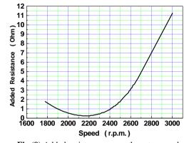
Fig.(9) Added resistance versus the rotor speed.
