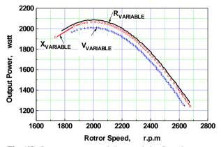
Fig. (13) Output power -speed characteristics for voltage, resistance and reactance variation.
