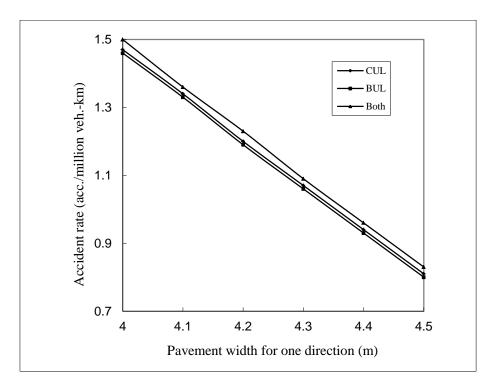
Figure (3): Relationship between Pavement Width and Accidents Rate for Undivided Highways
