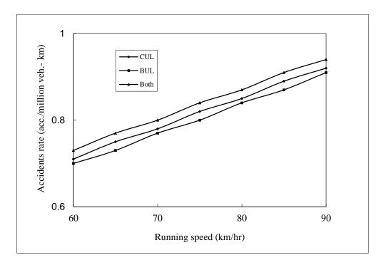
Figure (5): Relationship between Running Speed and Accidents Rate for Undivided Highways
