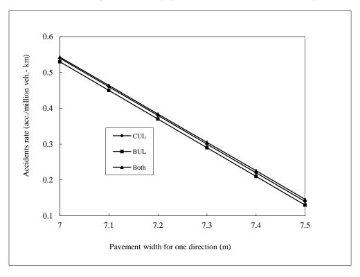
Figure (6): Relationship between Pavement Width and Accidents Rate for Divided Highways
