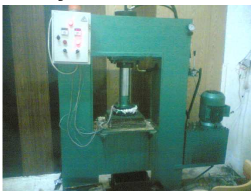
Fig. 3. Hydraulic pressing machine used for Manufacture of wood from agriculture waste (rice straw)
