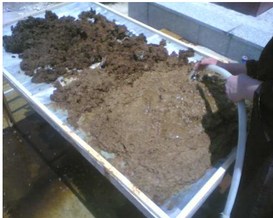
Fig. 4. Separating of salts, lignin and impurities from pulping
