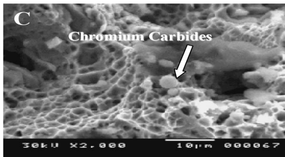
Fig.7 Fracture surfaces of tensile specimen after thermomechanical treatment
