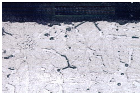
Fig. 7 Machined surface of Al 1050/15% SiCp ( V=28 rpm, \delta=0.25 mm, f=0.4 mm/rev, V_f=5\% , P_s=7.0\mu\text{m} ), (X200)
