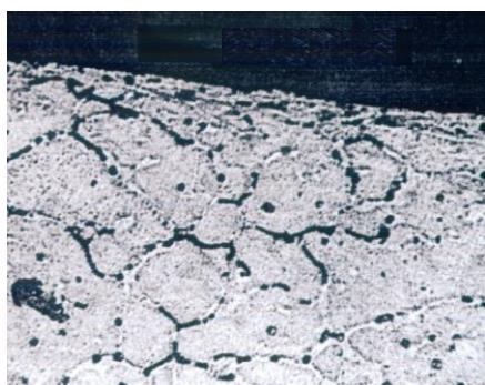
Fig. 9 Machined surface of Al 1050/ SiC ( V=90 rpm, \delta=1 mm, f=0.8 mm/rev, V_f=15\% , P_s=14\mu\text{m} ), (X200)
