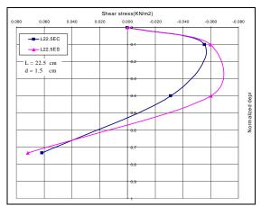
Fig. 8 Shear stress distribution along pile length for cases ( $L_{22.5}EC$  and  $L_{22.5}ES$ )
