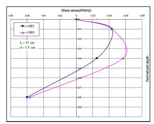
Fig. 7 Shear stress distribution along pile length for cases ( $L_{15}EC$  and  $L_{15}ES$ )
