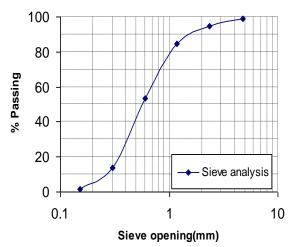
**Fig.2** Sieve Analysis test for the upper and lower sand layer
