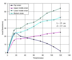
Fig. 5 Time- Axial strain curves of pile model  $(L_{25}E_S)$
