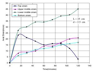
**Fig. 4** Time-Axial strain curves of pile model ( $L_{25}E_c$ )
