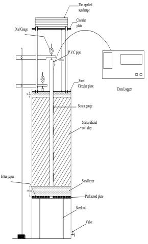
Fig. 1 The experimental rig
