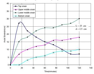
**Fig. 6** Time- Axial strain curves of pile model ( $L_{25}F$ )
