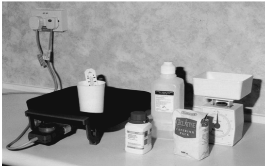
Fig. (1): Injection materials, from right to left: weighing scale, pack of gelatin powder, bottle of normal saline, box of lead oxide (PbO), thermostatically controlled frying pan as a water bath and 100gm of PbO in a mixing bowl with a thermometer respectively.
