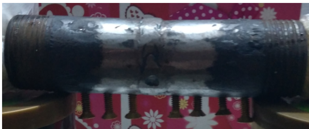
Fig. 4. Two pipe pieces after welding and filling with corrosive water S2 (seawater).
