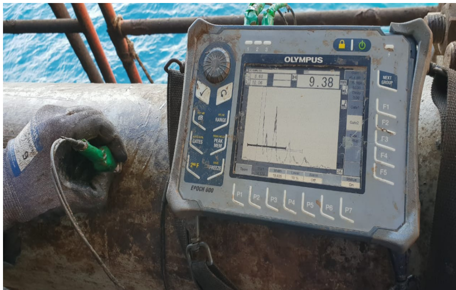
Fig. 6. Photo for example of using of OLYMPUS UT device to locate corroded area.
