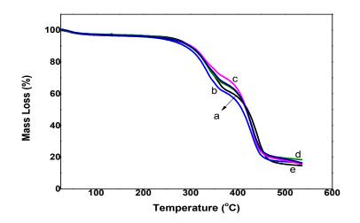
Fig. 3. TGA graphs blank furniture textile fabrics (a) F-CH-GMPP 20 (b), F-CH-GMPP 30(c), F-CH-GMPP 50 (d) and F-CH-GMPP 70(e).
