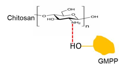
Fig. 5. Schematic diagram representing the interaction between GMPP and Chitosan chains
