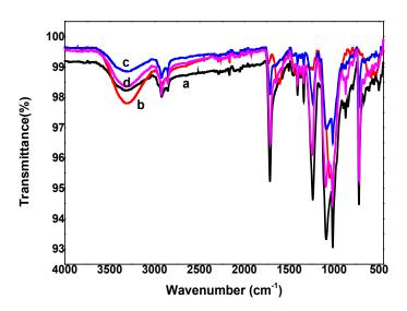
Fig. 4. FT-IR spectra of blank furniture textile fabrics (a) GMPP (b), F-CH-GMPP20(c), F-CH-GMPP70 (d).
