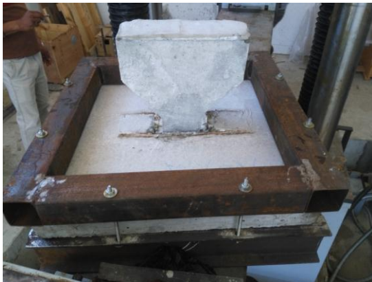
Figure (8): Preparing the slabs for testing
