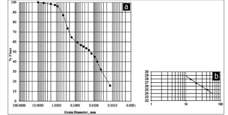
Figure (8) Shows  $\underline{\mathbf{a}}$ . grain size distribution curve for Dedan site,  $\underline{\mathbf{b}}$ . determination of Atterberg limits of soil
