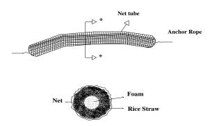
Fig. (1): Longitudinal and cross sections of rice straw barriers
