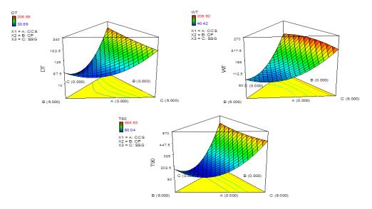
Figure (4): Response surface plot estimating the effect of CCS ( $X_1$ ), CP ( $X_2$ ) and SSG ( $X_3$ ) on the disintegration time (a), wetting time (b) and  $t_{90}$  (c) of vardenafil hydrochloride ODTs.
