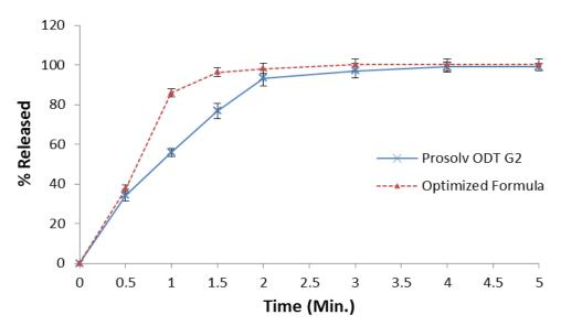
Figure (9): Dissolution profiles of vardenafil hydrochloride ODTs and Prosolv<sup>®</sup> ODT (a ready ODT system).
