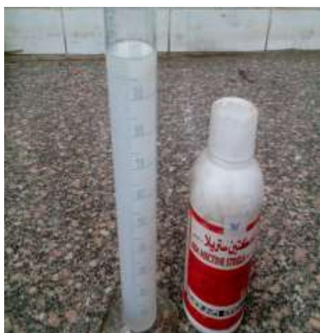
The emulsification test before and after storage doesn't conform to the specifications (Volume of Sediment/cream layer is more than 2 ml)
