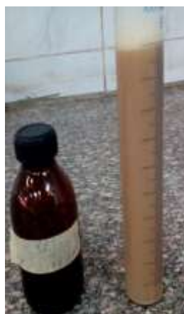
The emulsification test before conforms to specifications but after storage doesn't conform to specifications (Sample color changed) (Volume of Sediment is less than 2 ml)
