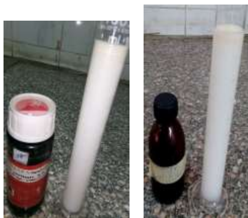
The emulsification test before and after storage doesn't conform to specifications (Volume of Sediment/cream layer is more than 2 ml)
