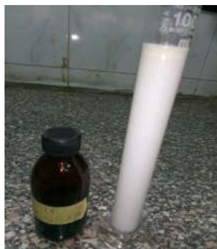
The emulsification test before and after storage doesn't conform to the specifications (Volume of Sediment/cream layer is more than 2 ml)
