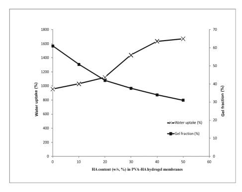
Fig. 1- Effect of HA content in PVA hydrogel membranes on gel fraction and water uptake(%).
