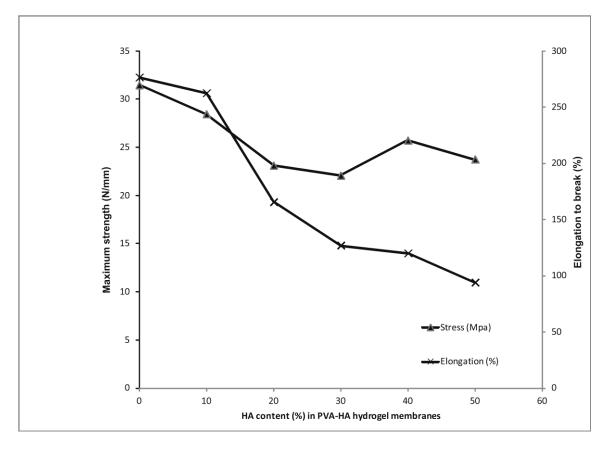
Fig. 2- Effect of hyaluronic acid contentes on mechanical properties of PVA hydrogel membrane.
