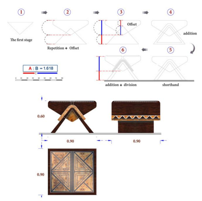
Figure 15 the main structural stages of the first model and the stages of generating the proposed design.
