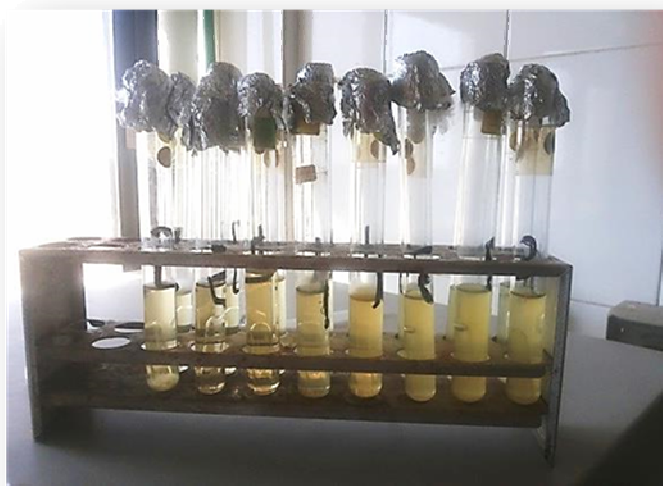
Fig. 2. The gas accumulation and yellow color in the Durham tubes in the presumptive test
