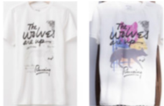
Figure (1) shows the form of interactive textile prints (Photochromic prints) before and after the effect (UV light). (Left to right)(6)
