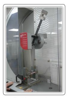
Fig. (1) Impact strength test.
