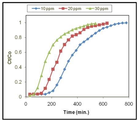
Fig. 4. Breakthrough curves of the effects of different conc. on biosorption of CR onto water hyacinth ( $\mathbf{F} = 1 \text{ ml min}^{-1}$ ,  $C_o = 20 \text{ mg } l^{-1}$ )
