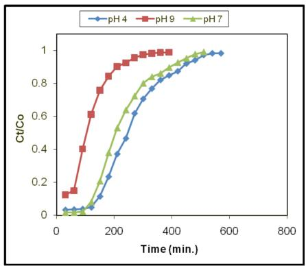
Fig. 1. Breakthrough curves of the effects of pH values on biosorption of CR onto water hyacinth ( $\mathbf{F} = 1 \text{ ml min}^{-1}$ ,  $C_0 = 20 \text{ mg } l^{-1}$ )
