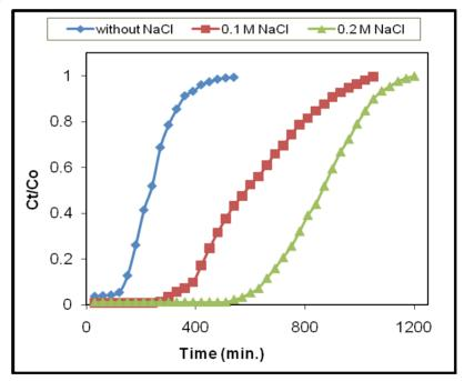
Fig. 5. Breakthrough curves of the effects of existing salt (NaCl) on biosorption of CR onto water hyacinth (  $\mathbf{F} = 1 \text{ ml min}^{-1}$ ,  $C_o = 20 \text{ mg l}^{-1}$ )
