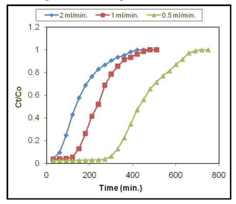
Fig. 2. Breakthrough curves of the effects of flow rates on biosorption of CR onto water hyacinth (  $\mathbf{F} = 1 \text{ ml min}^{-1}$ ,  $C_0 = 20 \text{ mg } l^{-1}$ )
