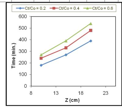
Fig. 7. Isoremoval lines for 0.2,0.4,0.6 breakthrough for different bed height  $(C_o=20~mg~l^{-1}~,~\textbf{F}=1ml~min^{-1})$
