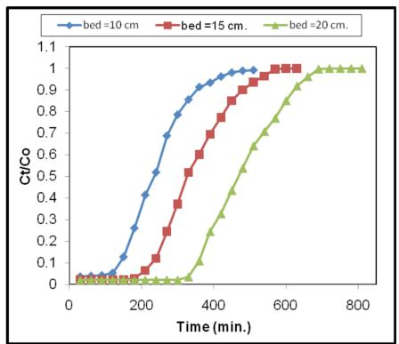
Fig. 3. Breakthrough curves of the effects of different bed depth on biosorption of CR onto water hyacinth ( $\mathbf{F} = 1 \text{ ml min}^{-1}$ ,  $C_0 = 20 \text{ mg l}^{-1}$ )
