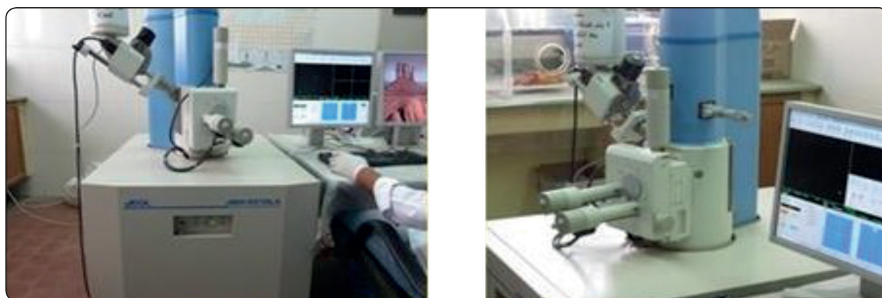
Fig. (2): Scanning electron microscopy –energy dispersive X ray analytical system (SEM-EDX).
