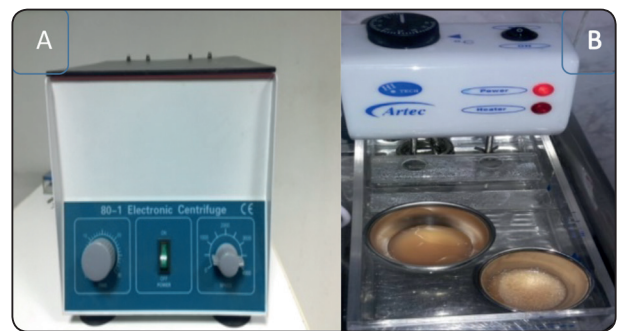
Fig. (2) Photograph of the centrifuge (A) and the hot water path containing a dish of preparation to be used as a membrane and the a second dish containing the PRGF mixed with Xenograft (B).
