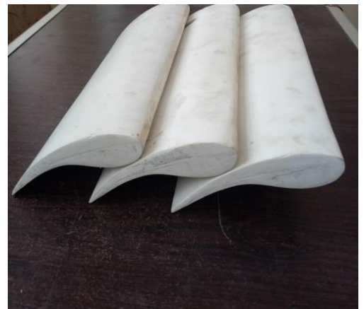
Fig.8 A photo of EN0005 blades with 0.16m chord length
