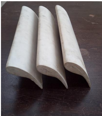
Fig.6 A photo of EN0005 blades with 0.12m chord length
