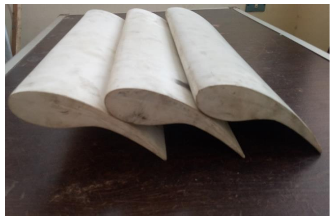
Fig.5 A photo of EN0005 blades with 0.18m chord length
