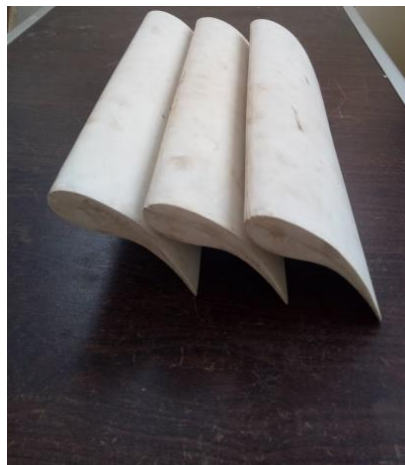
Fig.7 A photo of EN0005 blades with 0.14m chord length
