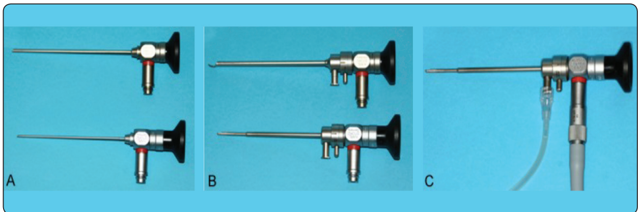
Fig. (8) Rigid endoscopic systems: A. Optics (Rigid) 2.7 mm and 1.9 mm. 30 degree view angle. B. Optic assembled with its support. C. Connection to the light source and irrigation. (24)
