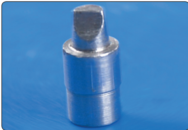
Fig. (2) The machined die with heavy chamfer preparation.
