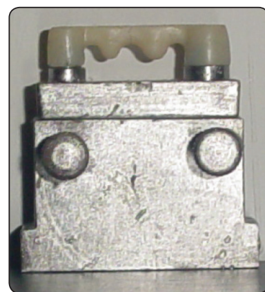
Fig. (1) Construction of provisional F.P.D for fracture resistance testing
