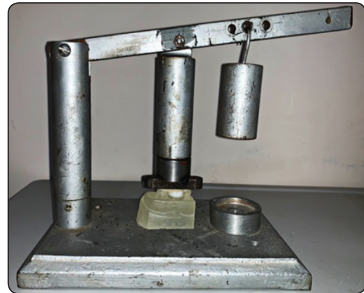
Fig. (6) An especially designed static loading device to ensure an effective flow of the cement and maximum adaptation during cementation.
