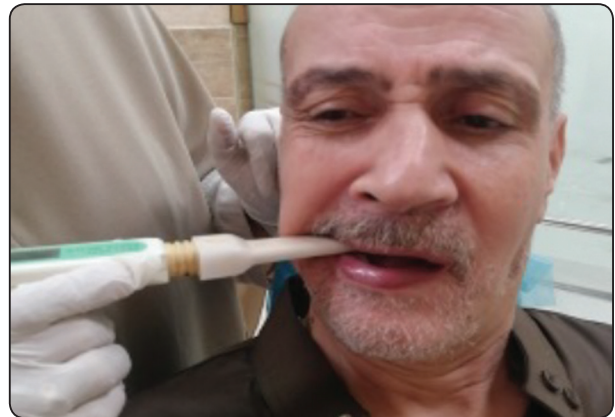
Fig. (6) Patient bite on the tip of the dispocap of the forcemeter with his maximum biting force.
