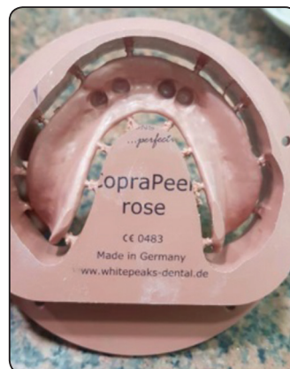
Fig. (3) PEEK resin milled overdenture base
