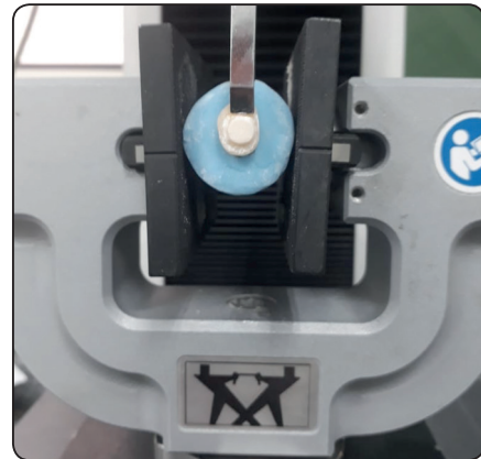
Fig. (1): The tested sample attached to universal testing machine
