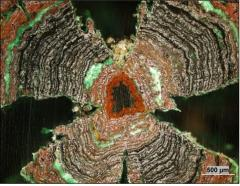
Figure (4) OM image of a needle in transversal section of a brass clips forged in torsade
