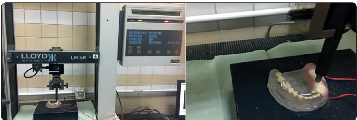
Fig. (4): Measuring the microstrains using strain gauges.
