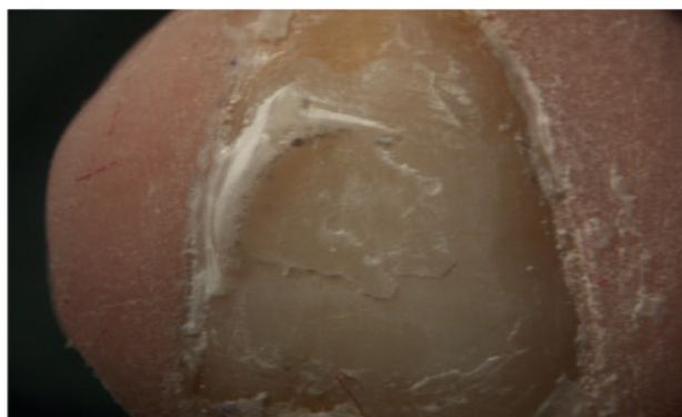
Cohesive failure within resin cement III
