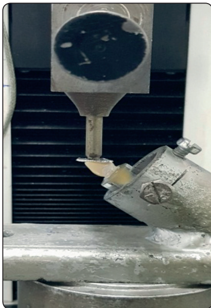
Fig. (4) Mounted sample loaded in the universal testing machine for mechanical testing.
