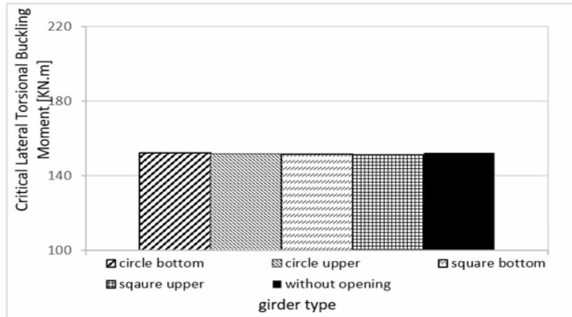
Figure 18 Lateral torsional buckling moment mode for all analyzed girders for case study (1)
