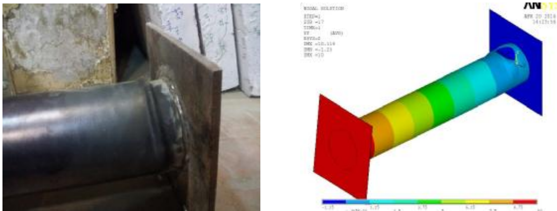
Figure 18: Failure mode shapes of CB1
