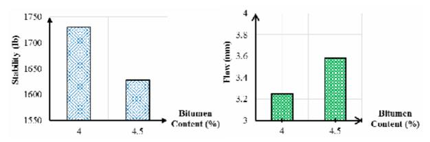
Figure (8): Effect of Bitumen Content on Marshall Stability and Flow for Open Mix (2C).
