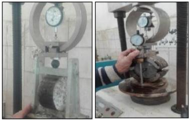
Figure (7): Marshall and Indirect Tensile Testing for Grouted Asphaltic Molds.
