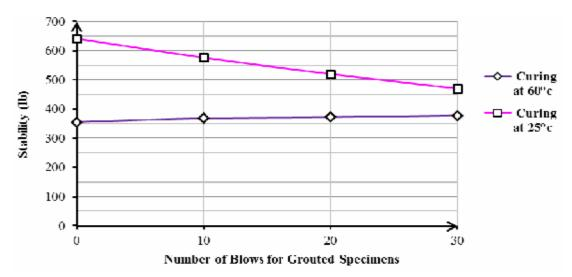
Figure (13): Effect of Curing Temperature Degrees on the Stability of SFP Specimens.
