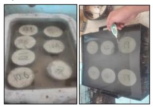
Figure (6): Grouted Asphaltic Molds during Curing Process.
