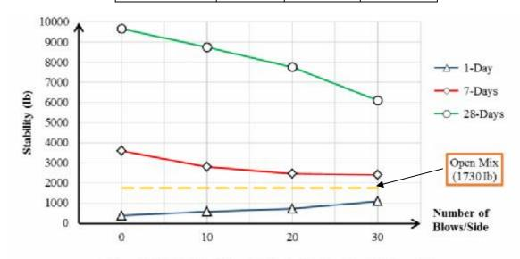
Figure (11):Stability of Grouted Asphaltic Moulds at Different Ages
