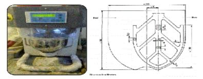
Figure (2): Grout Mixing Equipment and its Bowl and Blade.
