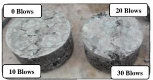
Figure (12): Failure Shape of Marshall Testing for Grouted Molds.
