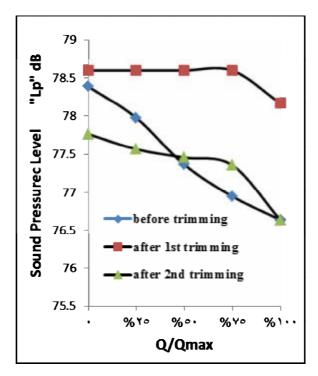
Fig. 25 Comparison between sound pressure level at original impeller diameter,  $1^{st}$ , and  $2^{nd}$  trimmed impeller at  $\varphi$ =270
