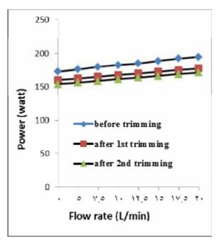
Fig. 11 (Ps-Q) curve of the pump at three impeller diameters
