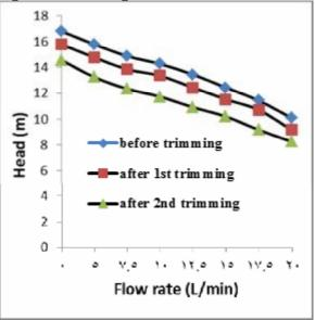
Fig. 10 (H-Q) curve of the pump at three impeller diameters
