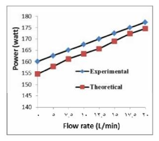
Fig. 15(Ps – Q) curve for theoretical and experimental results after trimming at "RPM=2850"
