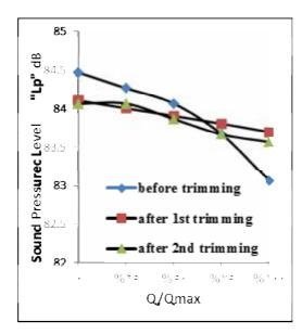
Fig. 23Comparison between sound pressure level at original impeller diameter,  $1^{st}$ , and  $2^{nd}$  trimmed impeller at  $\phi$ =90
