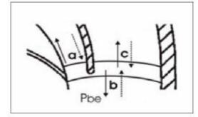
Fig. 20 Flow recirculation, discharged, and backed to pump [10]
