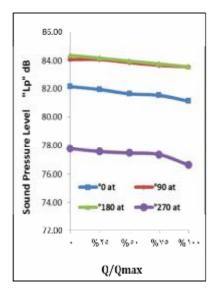
Fig.19 Sound pressure level at different flow rates and reference angles for trimmed impeller down to (104mm)
