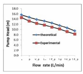
Fig. 14 (H - Q) curve for theoretical and experimental results after 2nd trimming at "RPM=2850"
