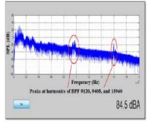
Fig.26Pressure pulsation at BPF and its harmonics at impeller diameter D=112mm
