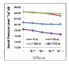
Fig. 17Sound pressure level at different flow rates and reference angles for untrimmed impeller
