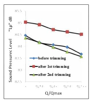
Fig. 24 Comparison between sound pressure level at original impeller diameter,  $1^{st}$ , and  $2^{nd}$  trimmed impeller at  $\varphi$ =180
