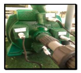
Fig. 2 Vocal microphones on pump casing
