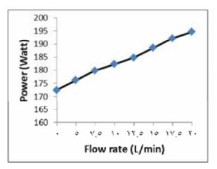
Fig. 7Pump Performance (Ps - Q) Curve at "2850 RPM"
