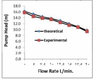
Fig. 13(H - Q) curve for theoretical and experimental results after 1sttrimming at "RPM=2850"
