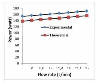
Fig. 16(Ps - Q) curve for theoretical and experimental results after 2ndtrimming at "RPM=2850"
