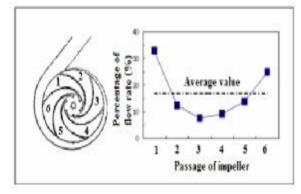
Fig. 21Flow rate distribution in all channels of the impeller [15]
