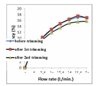
Fig. 12  $(\eta$ -Q) curve of the pump at three impeller diameters
