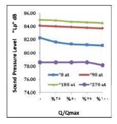
Fig. 18 Sound pressure level at different flow rates and reference angles for trimmed impeller down to "108mm" diameter
