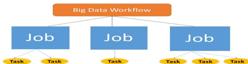
Fig. 1. Split job into tasks to assign on cluster nodes.
