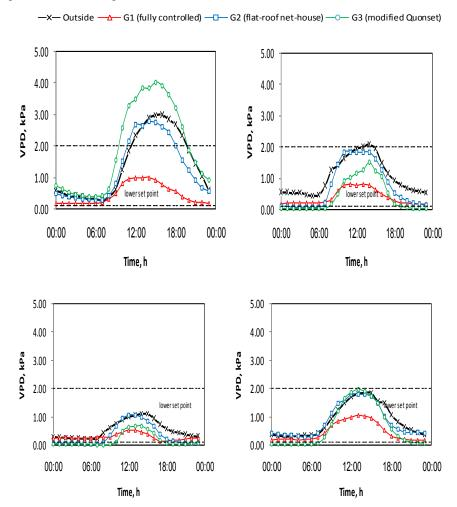
Fig. (4): Changes in vapor pressure deficit within the three greenhouses (G1, G2, and G3) as a function of time during summer (A), autumn (B),; winter(C), and spring (D).
