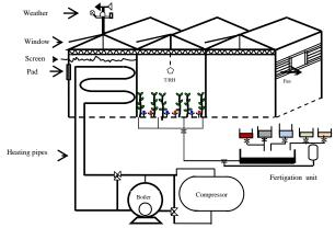
(a) Gable-even-span greenhouse (Multi-span)
