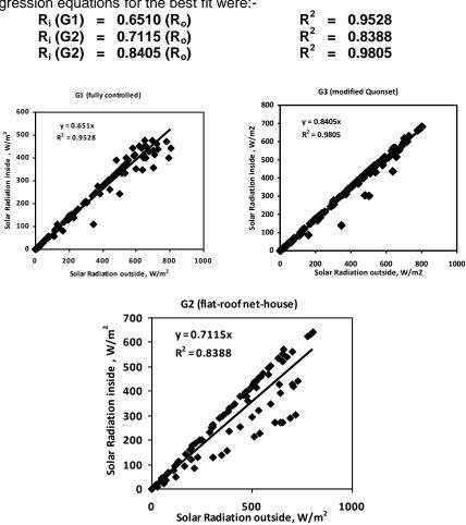
Fig (6): Solar radiation flux incident inside the three different structural forms of greenhouses (G1, G2, and G3) versus solar radiation flux incident outside.
