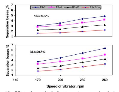
Fig. (2); Effect of speed of vibrator and rear angle of elevator on separation losses at different of moisture contents.
