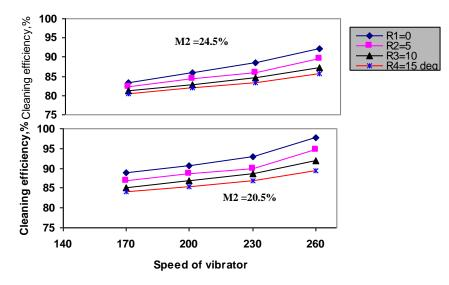
Fig. (4); Effect of speeds of vibrator and rear angle of elevator on cleaning efficiency at different of moisture contents.
