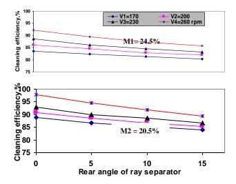
Fig. (3); Effect of rear angle of ray separator and speeds of vibrator on cleaning efficiency at different of moisture contents.
