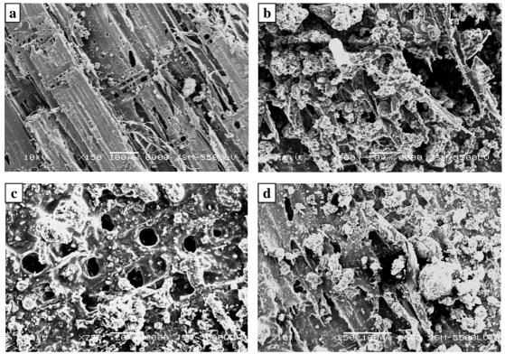
Figure (15) SEM images of the wood samples tested, shows <u>a</u> weakness and growing of microorganism on the wood surface. <u>b</u> Cellulose fibrils originating from mechanical disruption of the wood cells surface by the fungal attack, <u>c</u> degraded pit membranes were observed in the inner part, <u>d</u> crystallized dehydrate calcium sulfate was found inside
