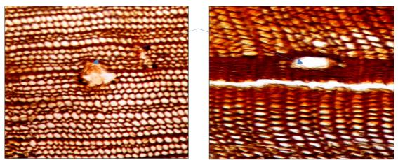
Figure 17 (a, b) transversal section of wood sample, shows resinaceous aperture which characteristic the halepensis pine.
