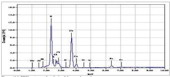
Figure (16) EDX patterns of analysis of the wood sample.
