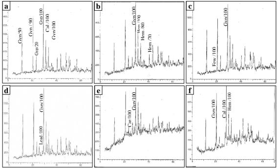
Figure (11) XRD pattern of the paint layers of Qaitbay's madrassa ceiling  $\underline{\mathbf{a}}$  white pigment  $\underline{\mathbf{b}}$  red pigment  $\underline{\mathbf{c}}$  blue pigment  $\underline{\mathbf{d}}$  brown pigment  $\underline{\mathbf{e}}$  black pigment  $\underline{\mathbf{f}}$  gilded layer.
