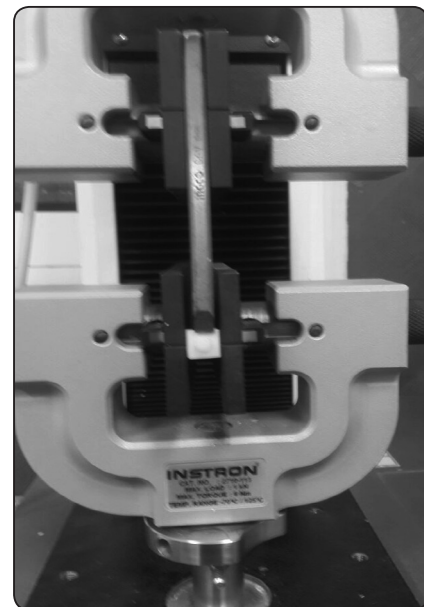
Fig. (3) Bonded specimen mounted in the universal testing machine
