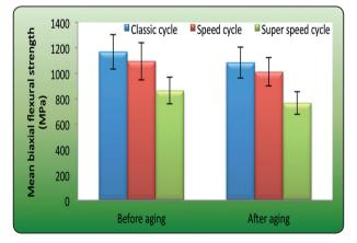
Fig. (5): Mean and standard deviation values of biaxial flexural strength in the different groups
