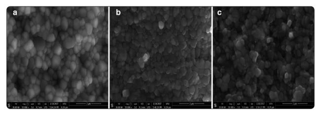
Fig. (6) : SEM images of zirconia samples sintered by A: classic, B: speed and C: super speed cycles without thermodynamic aging and before fracture showing the different grain patterns at 50000× (Top views)
