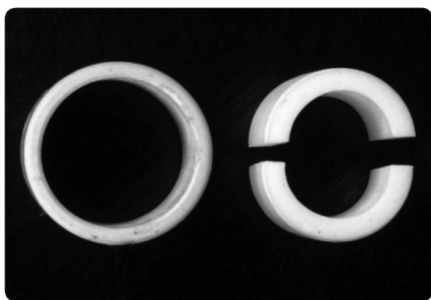
Fig. (2) Mold for composite samples fabrication.
