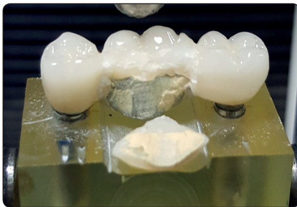
Fig. (3) Fractured implant supported metal ceramic bridges with CAD/CAM fabricated frameworks showed cohesive fracture within the porcelain
