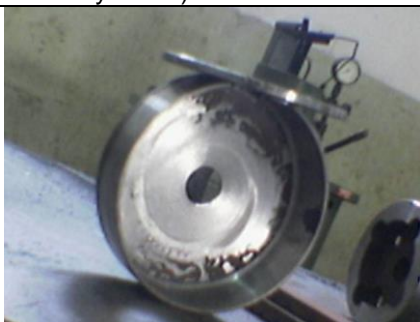
Fig. 7b: A Complete installation of brush metering device
